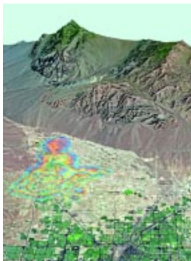
Figure 4. Subsidence zone near Las Vegas, NV. Developed by NPA Group, Kent, UK and published in Professional Surveyor.
