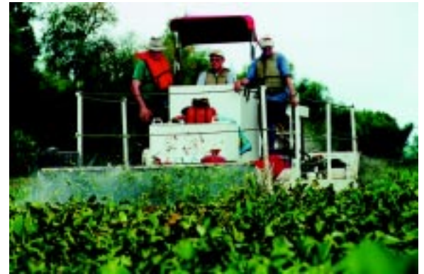
Figure 2. Mechanical control of invasive aquatic plants using the AquaSolutions' AquaTerminator machine.
