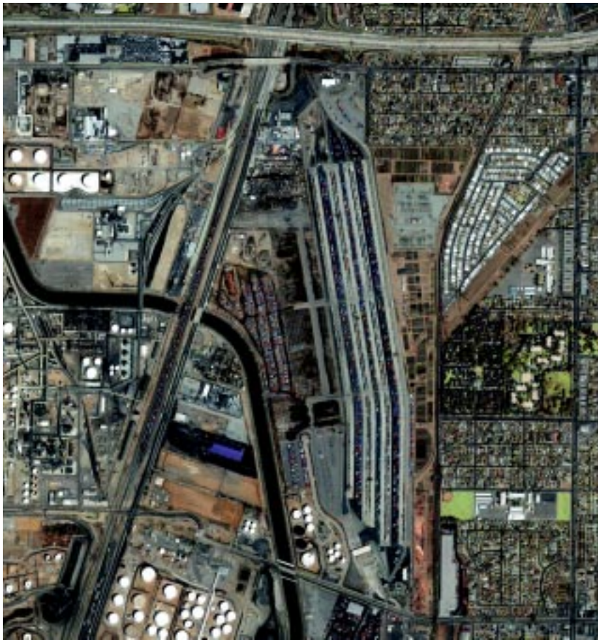
Figure 1. Carson intermodal connection yards. Simulated 1 meter resolution produced through convolution of 4m Ikonos RGB and 1m panchromatic.
