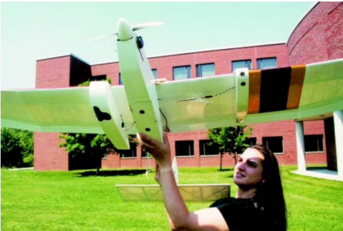
Figure 1. Bottom view of MAV showing remote sensing pods under wing.
