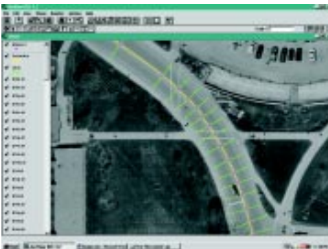
Figure 1. Centerline geometry extracted from aerial photograph.
