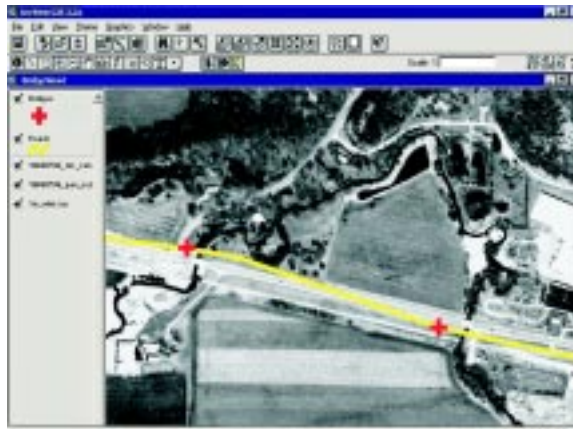
Figure 1. Bridge locations inferred from DOT linearly referenced records (red) can be inaccurate. Error in road centerline (largely the cause of the inaccuracy) is also apparent.
