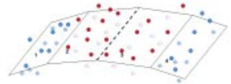
Figure 2. Regression Plane fitted to a cloud of LIDAR points.
